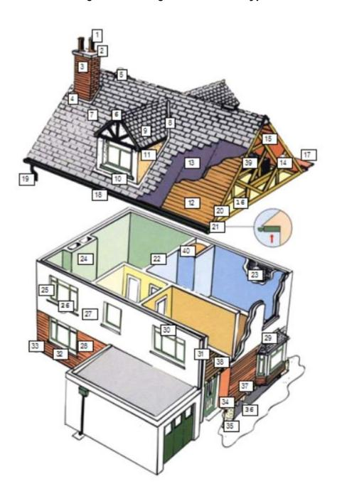
8 Valley guttering 9 Dormer projection Dormer flashing 10 Dormer cheeks 11 12 Sarking Roof felt 13 Trusses 14 15 Collar 16 Insulation 17 Parapet gutter Eaves guttering 18 Rainwater downpipe 19 20 Verge boards / skews 21 Soffit boards 22 Partition wall Lath / plaster 23 24 Chimney breast 25 Window pointing Window sills 26 27 Rendering Brickwork / pointing 28 Bay window 29 30 Lintels 31 Cavity walls / wall ties
